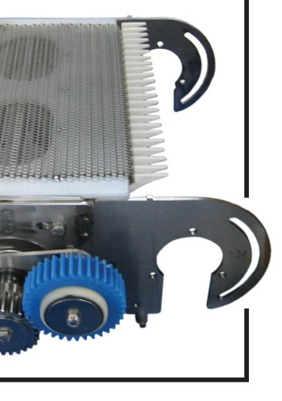
Our Transpositor **provides right-angle product transfers** and allow product lanes or patterns to be built across the width of receiving conveyors. The transfer function uses our sprocket-driven Microspan Chain. Servo or AC motor can power the depositing function.
